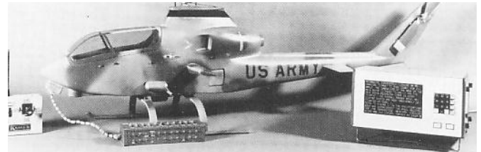
Fig. 4. COBRA Scale-Model Used for LOGMOD Tests LOGMOD. Because of the ability to store extensive logic information on small floppy disc units, the entire BRD-7 system logic can be contained within the LOGMOD unit.
